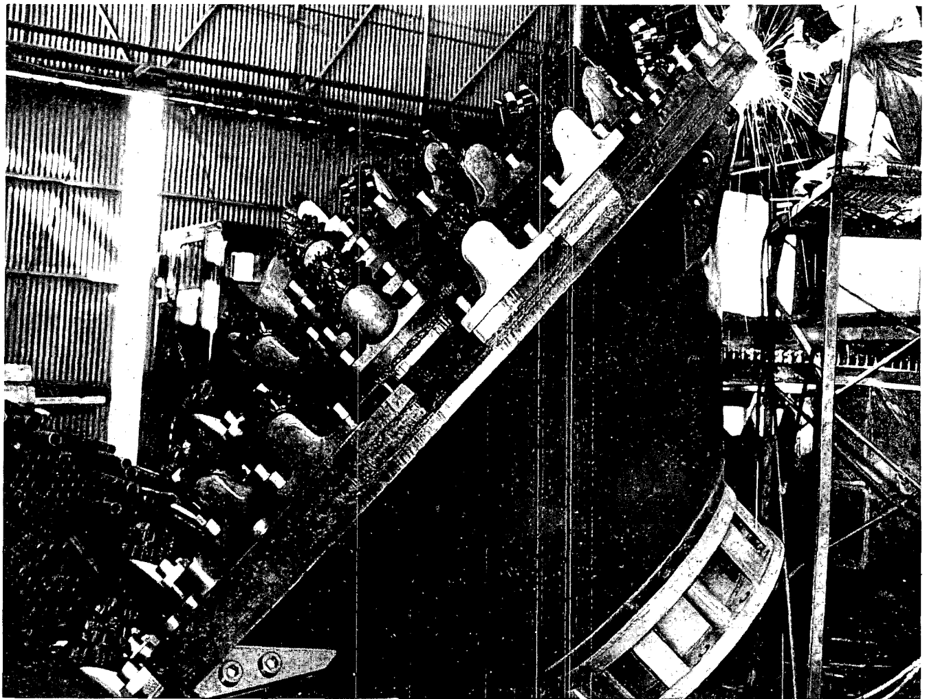
Fig. 8. View of a plate type large diameter drill bit. Photo-Hughes Tool Company.
